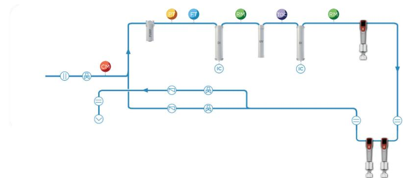
■ Flow transmitter    ■ Resistivity transmitter    ■ TOC indicator    ■ Solenoid valve    ■ Intelligent chip    ■ Drain
