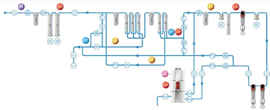
PS Pressure switch FT Flow transmitter LS Level sensor SV Solenoid valve IC Intelligent chip DCV Decompression valve D Drain
