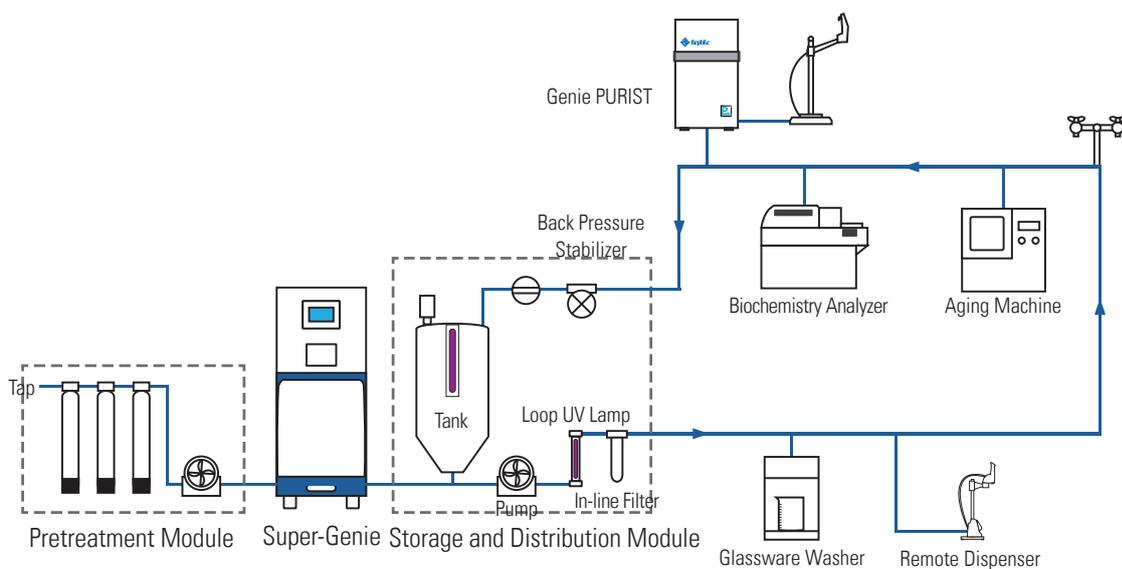
Super-Genie is designed to intergrate centralized water purification system together: from feed water prefiltration devices to distribution loop
